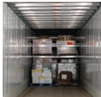
Same palletized cargo loaded with Kaptive Beam
