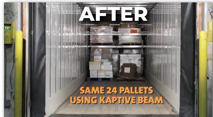
Kinedyne Kaptive Beam Double Decking Solution address' driver shortage problems and other hurdles truckers must face. By doubling a trailer's capacity you can deliver the same freight volumes with half the number of drivers.
